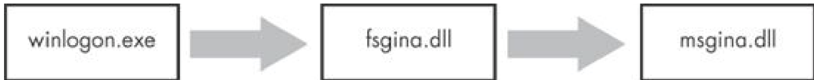
Figure 12-2. Malicious fsgina.dll sits in between the Windows system files to capture data.
